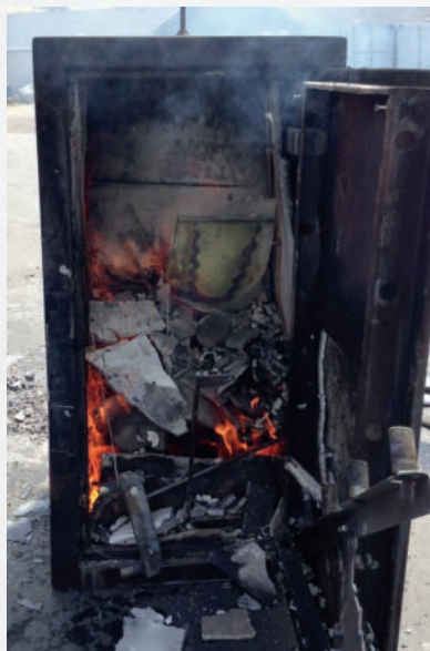
Leading competitor safe with 1-7/8" thick insulation after 90 minutes at 1680°.
